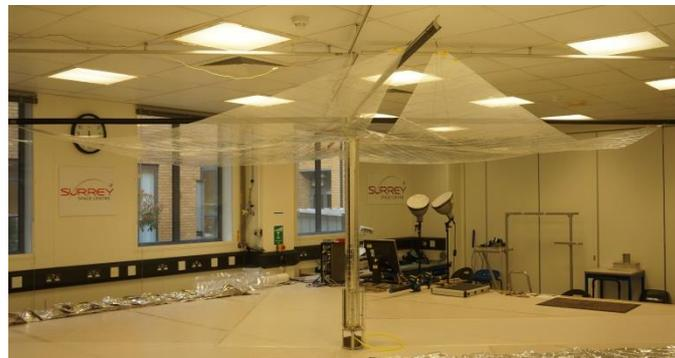
Fig. 5. InflateSail Inflatable Mast and Drag Sail Deployment Test
