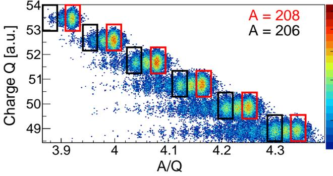
Figure 2: Two-dimensional identification matrix obtained with the VAMOS++ spectrometer. Nuclei with atomic mass number  $A = 206$  and  $A = 208$  are highlighted for several charge states measured in the spectrometer. Due to the low velocity of the recoils, an element identification ( $Z$ ) is not possible.
