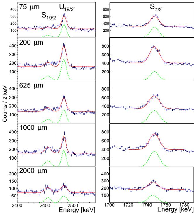
Figure 4: Doppler corrected  $\gamma$ -ray spectra for mass  $A = 207$  as a function of the target-to-degrader distance. Left: the  $19/2^- \rightarrow 13/2^+$  transition in  $^{207}\text{Pb}$ . Right: the  $7/2_1^- \rightarrow 5/2_1^-$  transition in  $^{207}\text{Pb}$  used for normalization.
