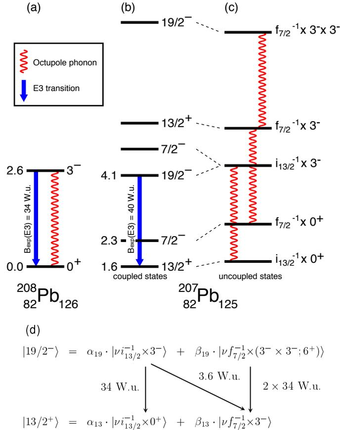
Figure 1: Illustration of the particle-octupole-vibration coupling model: (a) The lowest octupole-vibrational phonon of  $^{208}\text{Pb}$ , (b) selected states resulting from the particle-octupole-vibration coupling in  $^{207}\text{Pb}$ , (c) uncoupled (unperturbed) states in  $^{207}\text{Pb}$ , (d) wave functions of the  $13/2^+$  and  $19/2^-$  states in the particle-octupole-vibration coupling model. The energies of the known states are given in MeV.
