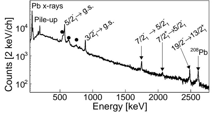
Figure 3:  $\gamma$ -ray spectrum gated on mass  $A = 207$  at the target-to-degrader distance of  $75 \mu\text{m}$ . The transitions marked with a circle correspond to the Coulomb excitation of the  $^{100}\text{Mo}$  target, Doppler corrected using the velocity vector of the heavy partner.
