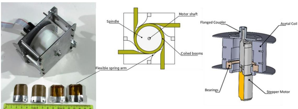
**Figure 6. Mechanism used for the deployment of the solar arrays in the prototype**
