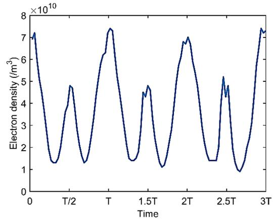
**Figure 1. Electron density variation during three orbital periods (IRI-2016, 2001, 1<sup>st</sup> March, altitude = 1000km, 85° inclination, T = 1 period, starting at 12h00UT, 0°N, 0°W)**
