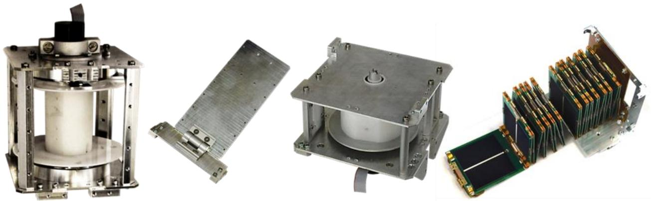
**Figure 4. Different manufactured parts of the prototype: EDT booms deployment mechanism, structure side panels, deployment mechanism used for the deployment of the solar arrays, Z folded deployable solar arrays**
