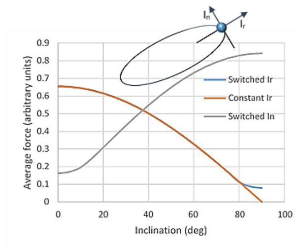
**Figure 2. Average drag force per orbit (arbitrary units) for horizontal and vertical tethers as a function of the orbit inclination (1000km altitude)**
