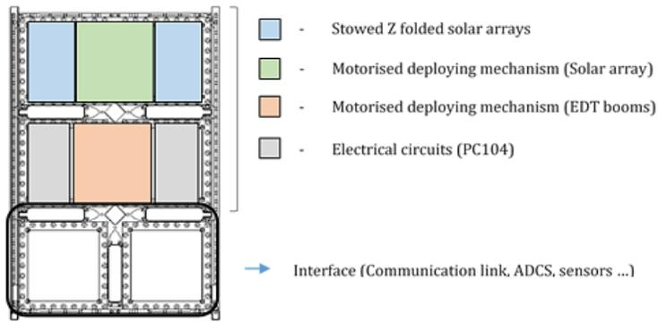
**Figure 5. Location of different prototype subsystems inside the 6U structure**
