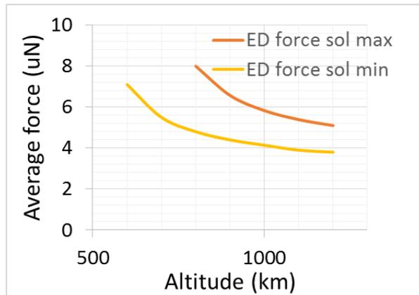
**Figure 3. Average force which can be obtained with the proposed propellant-less system as a function of altitude (for different solar activities 2002 vs 2008, equatorial orbits)**
