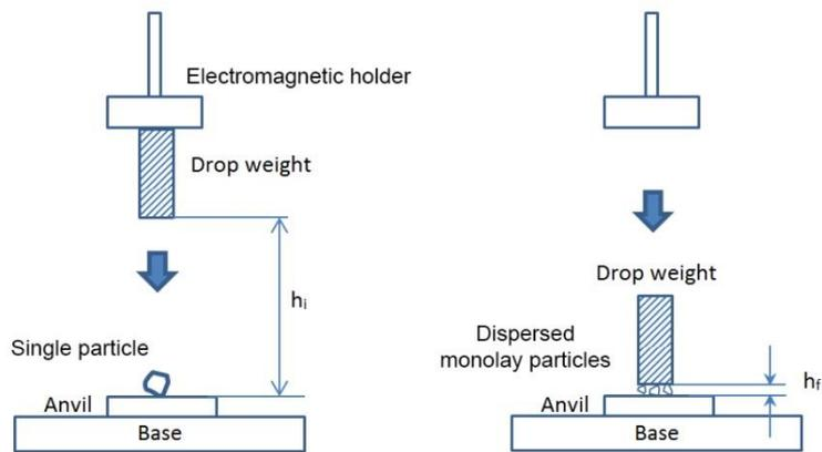
Fig. 2. Schematic diagram of Mini JK Drop Weight Tester and breakage energy calculation
