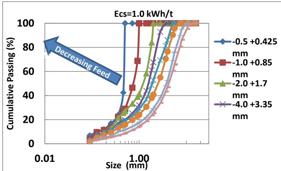
Fig. 5. Product size distribution of  $E_{cs}=1.0$  kWh/t at different original feed size X
