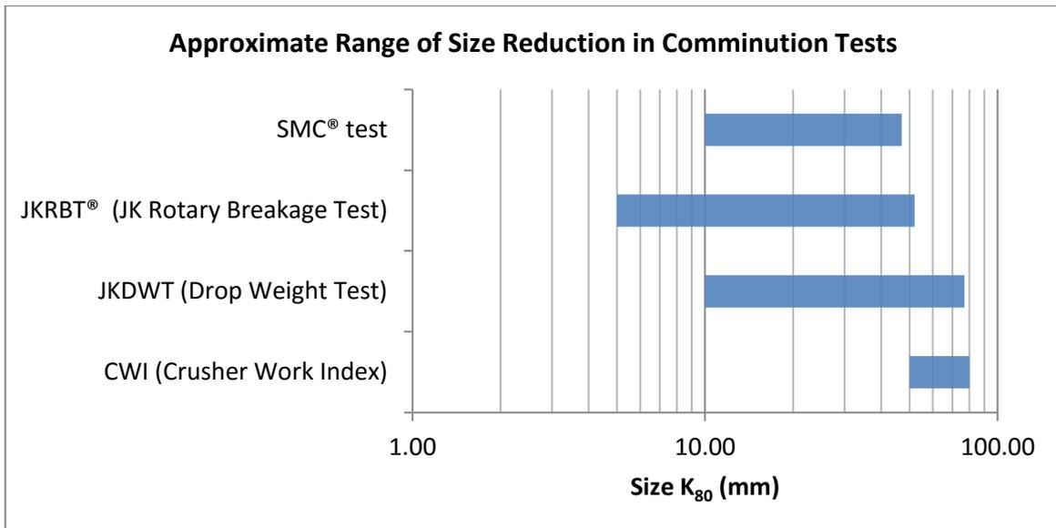
Fig. 1. Approximate range of size reduction in comminution tests
