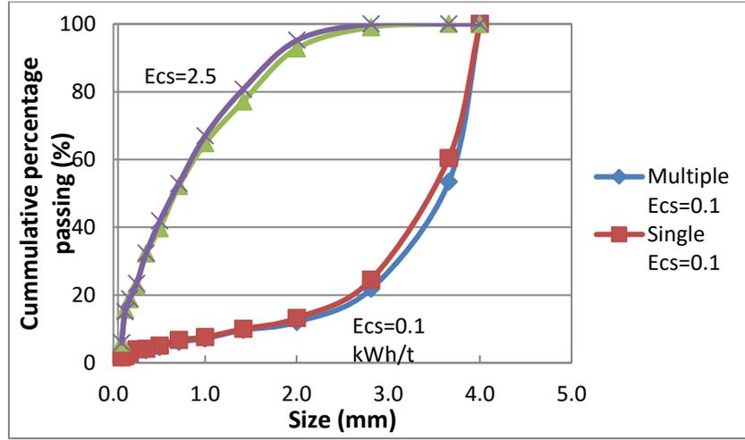
Fig. 6. Comparison between the single particle breakage and the monolayer multi-particle bed breakage for size fraction -4+3.35 mm
