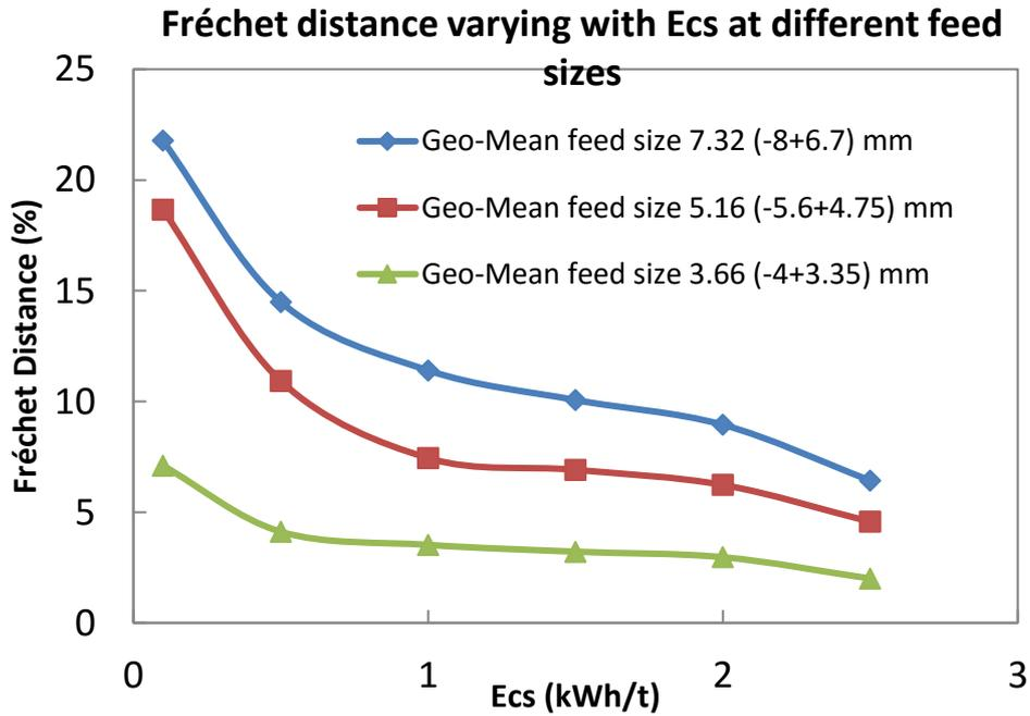
Fig. 8. Fréchet distance curve comparison between different feed sizes
