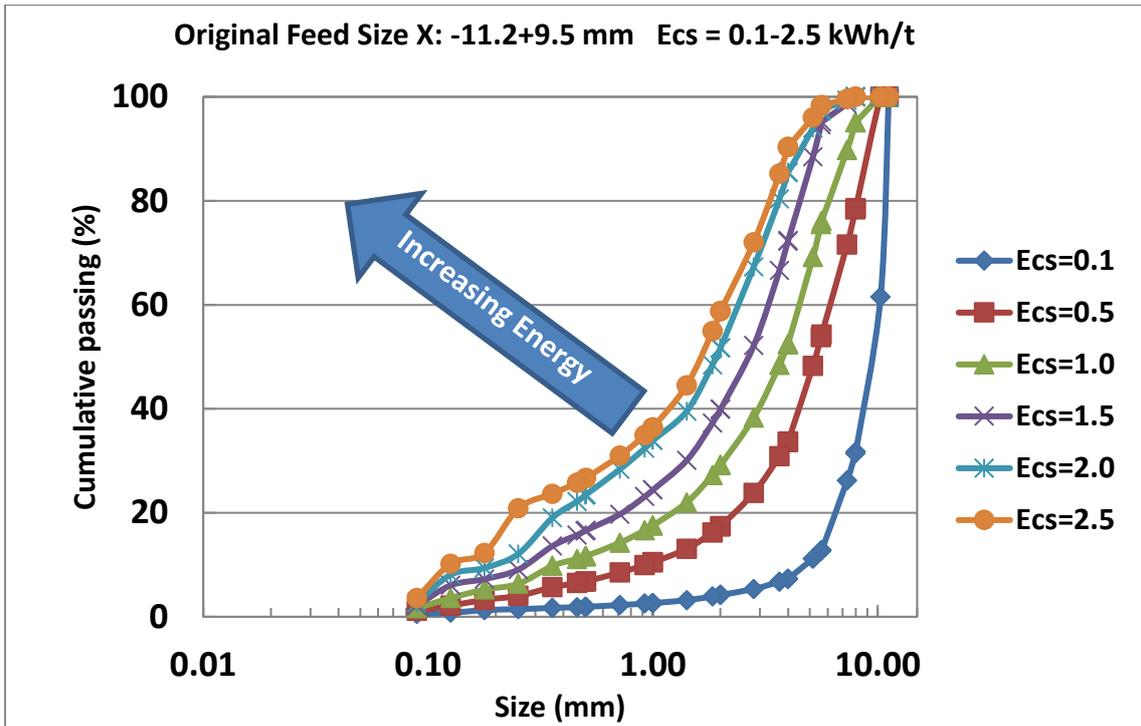
Fig. 4. Product size distribution of X= -11.2+9.5 mm at different Ecs
