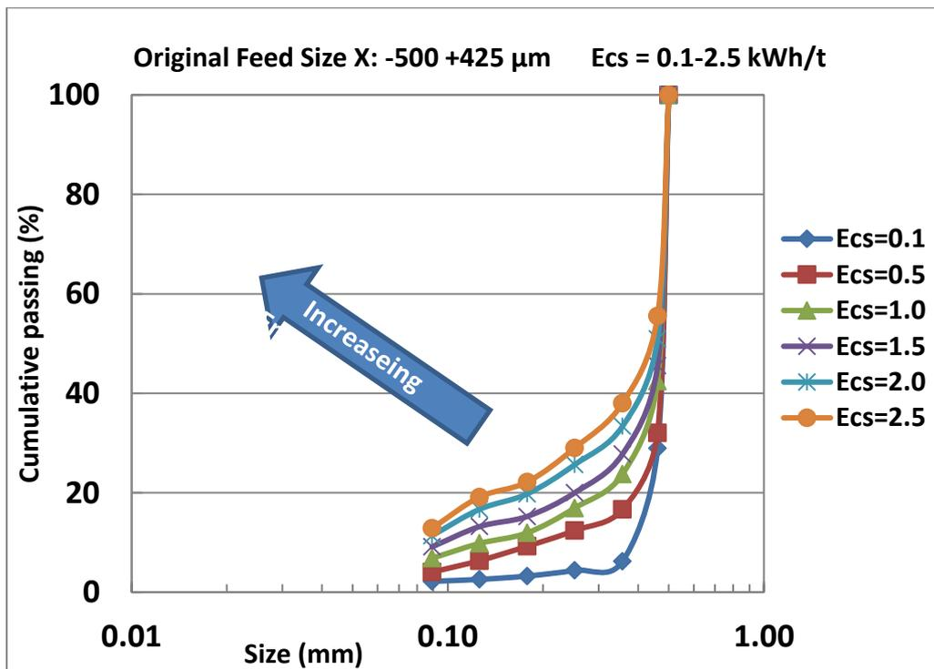
Fig. 3. Product size distribution of X= -500+425  $\mu$ m at different Ecs
