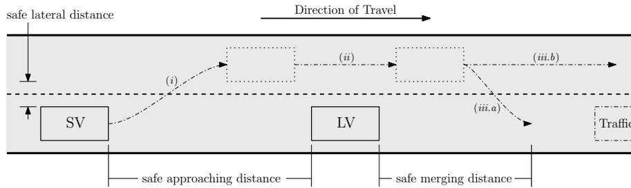
Figure 1: Basic schematic of an overtaking manoeuvre. **Note:** Different sub-manoeuvres are (i) lane-change; (ii) pass lead vehicle; (iii.a) merge back into original lane; (iii.b) continue in faster lane to pass traffic
