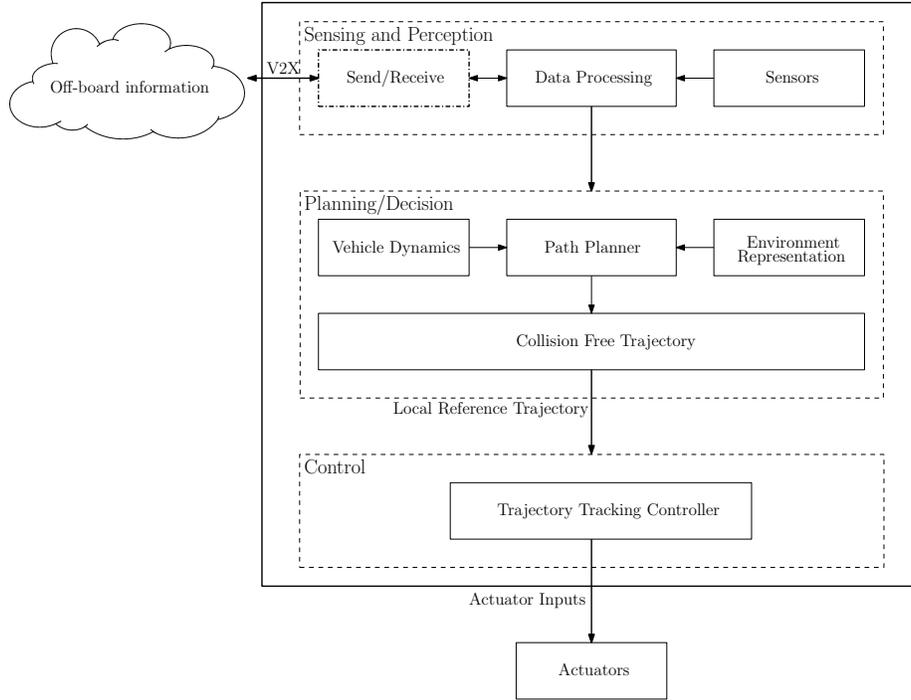
Figure 3: Overview of an autonomous driving system
