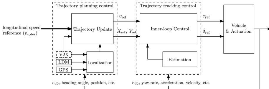
Figure 4: General control architecture for an autonomous vehicle [38, 43, 49–51]. (V2X block with dot-dash boundary: optional functionality)
