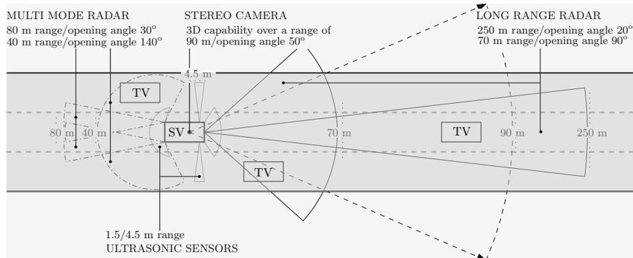
Figure 2: Visibility of an autonomous vehicle. **Note:** SV: Subject Vehicle, TV: Traffic Vehicle. Sensor performance specifications are based on [34]
