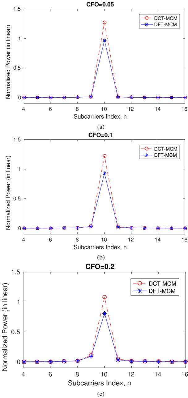
Fig. 5. Power spectrum (in linear) on the 10th subcarrier for DCT-MCM and DFT-MCM systems.(a) $\Delta fT=0.05$ . (b) $\Delta fT=0.1$ . (c) $\Delta fT=0.2$ .
