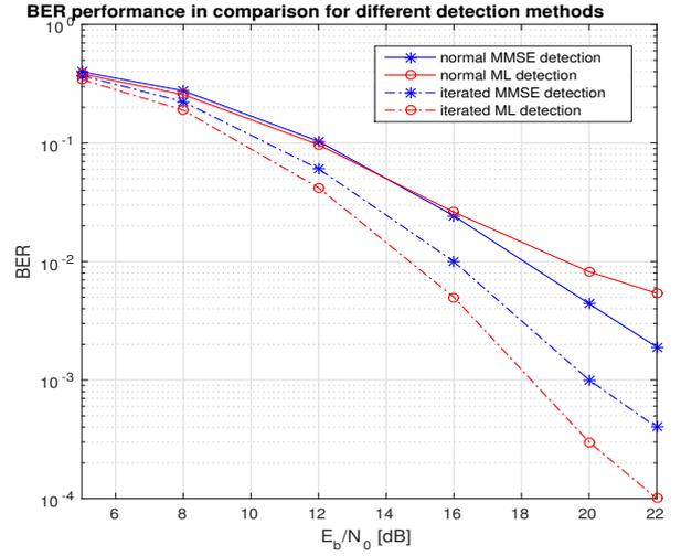
Fig. 7. BER performance for 8ASK DCT-MCM in normal and iterative detection methods in the presence of imperfections.
