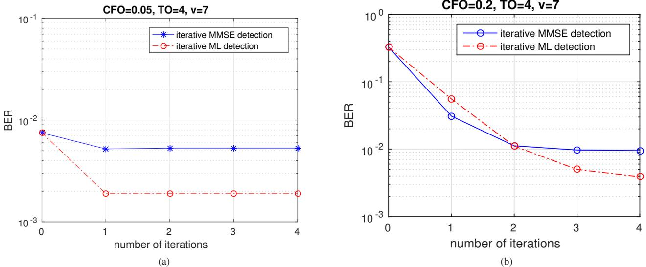
Fig. 8. BER performance at  $E_b/N_o=16\text{dB}$  for MMSE and ML detections for 8ASK DCT-MCM in the presence of imperfections (a) CFO=0.05, TO=4,  $v=7$ . (b) CFO=0.2, TO=4,  $v=7$ .
