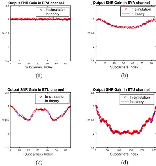
Fig. 3. The output SNR gain achieved in three typical channels. (a) EPA  $N=64$ . (b) EVA  $N=64$ . (c) ETU  $N=64$  (d) ETU  $N=256$ . [24].
