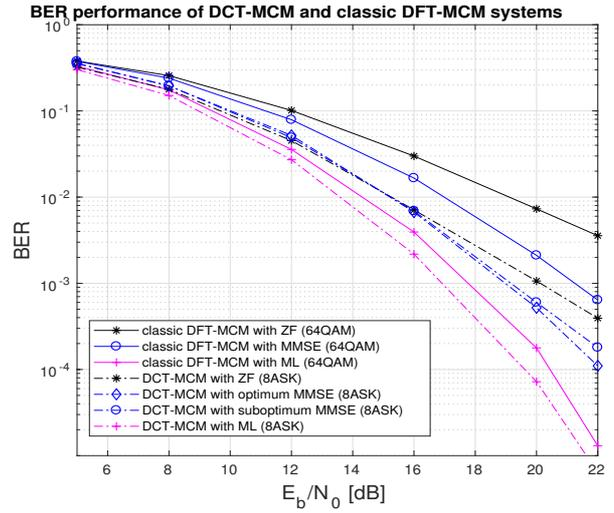
Fig. 4. BER performance for DCT-MCM and DFT-MCM systems in three detection methods
