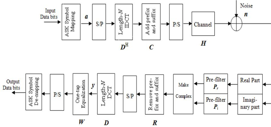
Fig. 1. Baseband system model for pre-filtering DCT-MCM systems
