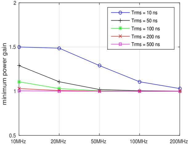
Fig. 2. The minimum signal power gain for different sampling frequency and RMS delay in a typical IEEE 802.11 channel.
