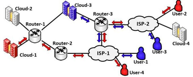
Figure 1. An example network architecture diagram of an ITV distribution system. Four users in two social user groups connect to two ISPs where Cloud-1 and Cloud-3 act as the media processing nodes.
