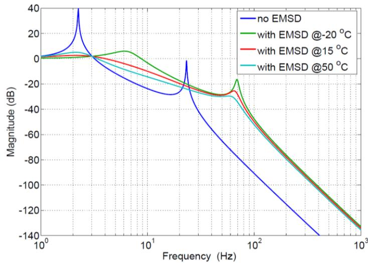
Fig. 3. Comparison of the force transfer functions between the system without EMSD and the system with EMSD at three different temperatures
