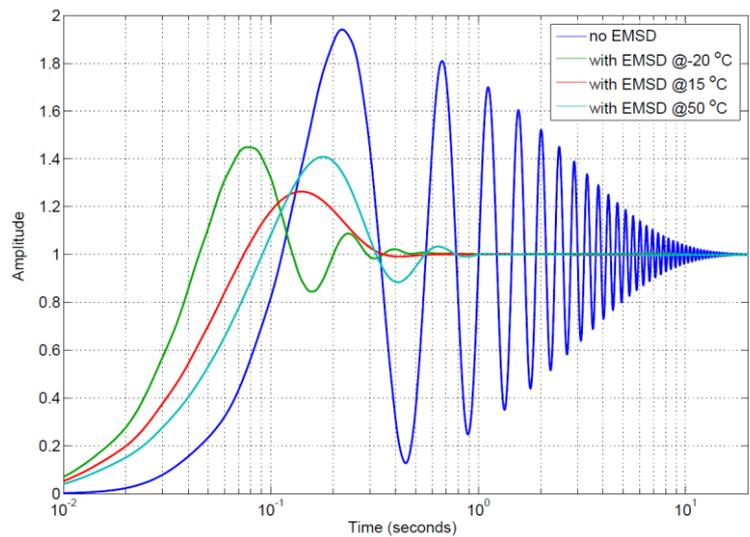
Fig. 4. Comparison of the step responses between the system without EMSD and the system with EMSD at three different temperatures
