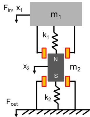
Fig. 2. Schematic representation of the 2-collinear-DoF model
