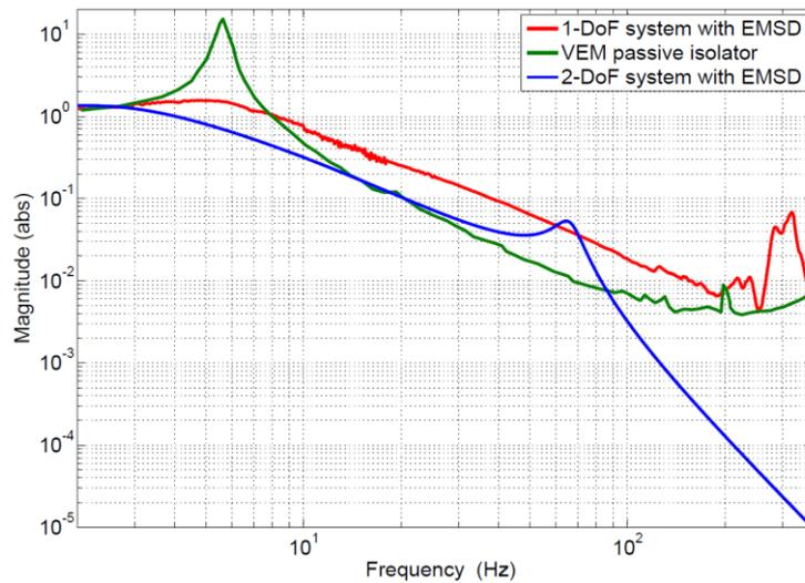
Fig. 5. Comparison of the force transfer functions between three different damping systems: (red) test result from 1-DoF system with EMSD [6]; (green) test result from VEM passive isolator [7]; (blue) analytical data from 2-collinear-DoF system with EMSD at 15°C
