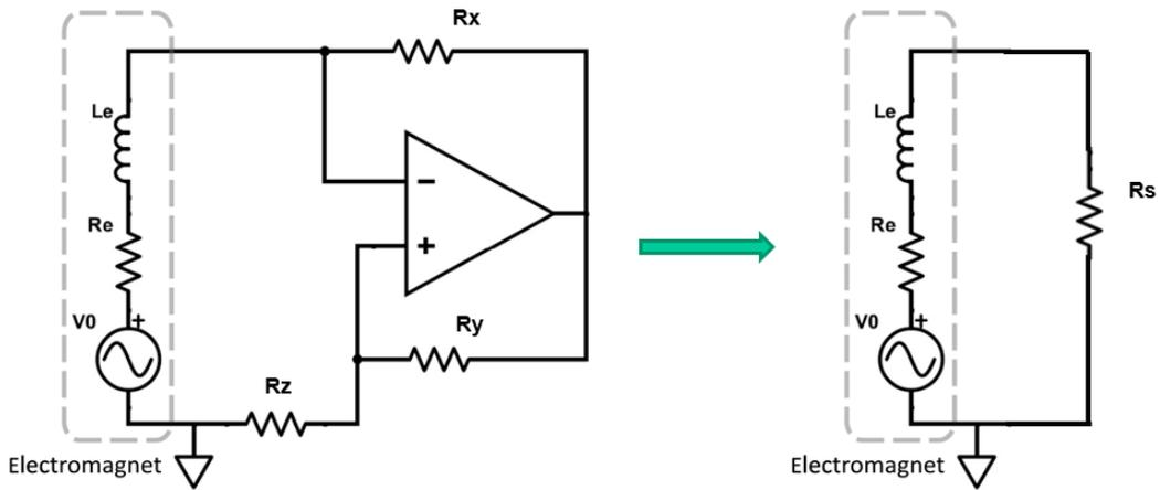
Fig. 1. Left-hand-side: electrical schematic of the negative resistance converter connected to the electromagnet. Right-hand-side: the equivalent circuit schematic where the negative resistance is represented by a passive resistor having negative magnitude.
