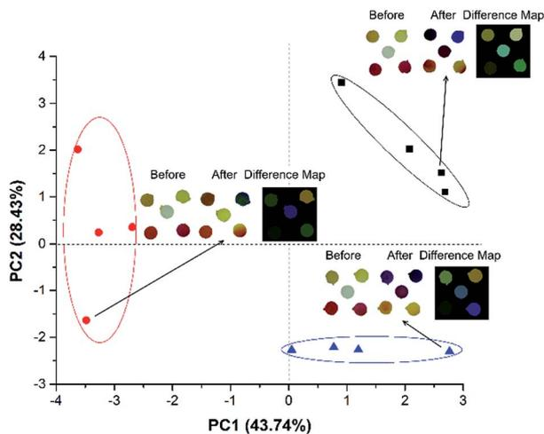
Fig. 4 PCA scores plot obtained from the *RGB* values extracted from the coloured membranes with 5 pH indicators in contact with volatile phase collected from a chamber containing meat contaminated with: ■ – isobutylamine; ● – triethylamine and ▲ – isopentylamine. High-lighted images show the real images of the colour changes profile of the sensor array for one of the experiments before and after the meat is contaminated with each amine and respectively difference map for each experiment.
