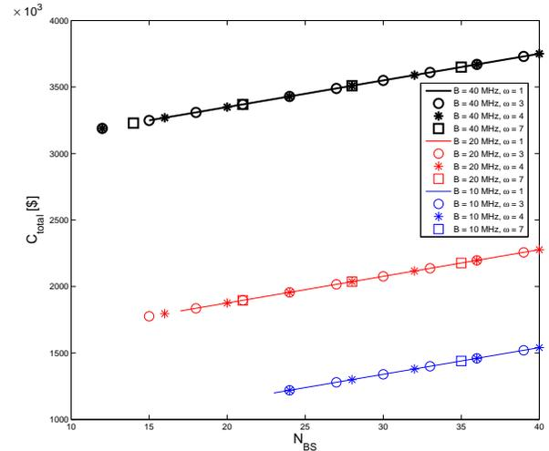
Figure 2. Total network costs for  $\mathcal{R}_{\text{area}} = 20$  Mbps/km<sup>2</sup>, and different frequency reuse factors and available bandwidth as function of the number of BSs.
