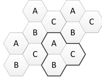
Figure 1. Cellular system employing reuse of frequencies.
