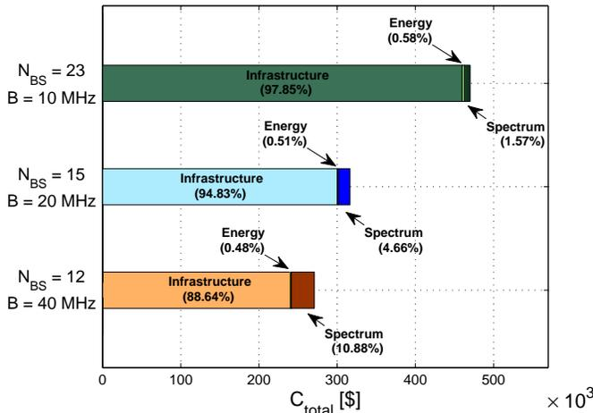
Figure 6. Detailed network costs per coverage area for  $\mathcal{R}_{\text{area}} = 20$  Mbps/km<sup>2</sup>, and the minimum number of BSs for  $B = 20$  MHz and  $B = 40$  MHz considering 100 coverage areas.
