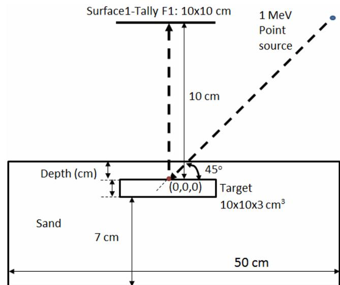
Fig. 2. The geometrical set-up of the MCNP5 simulation
