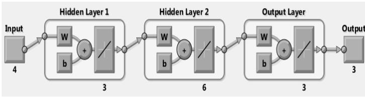
Fig. 6. The feedforward backpropagation structure of ANN1 for material classification.  $w$  is weight and  $b$  is bias.
