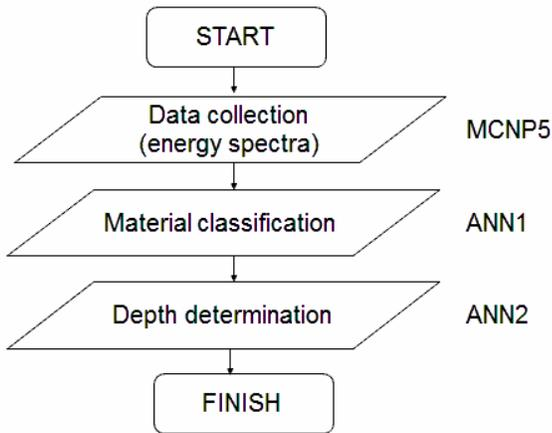
Fig. 1. Flowchart of the work on material classification and depth of the buried material
