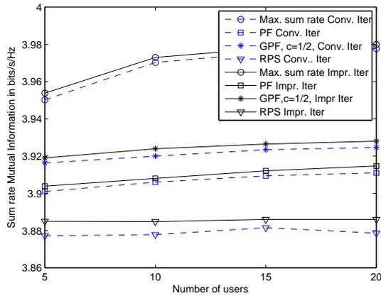
Fig. 4. Performance comparison of the MI based scheduling algorithms for the improved and conventional iterative IC-MMSE schemes for the QPSK system with  $2 \times 2$  antenna setup. All the curves are plotted at the 3rd iteration when the systems reach convergence, SNR 30 dB.
