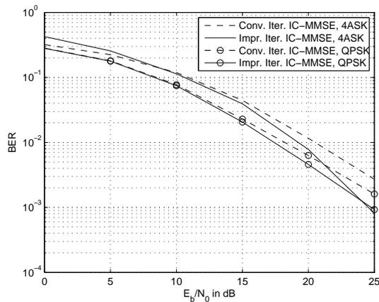
Fig. 6. BER performance of improved iterative receiver schemes with  $2 \times 2$  antenna setup. All the curves are plotted at the 3rd iteration when the systems reach convergence.
