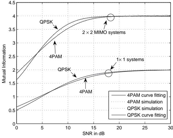
Fig. 1. Mutual Information versus received SINR for uncoded  $1 \times 1$  and  $2 \times 2$  MIMO systems with QPSK signaling and with 4ASK signaling.
