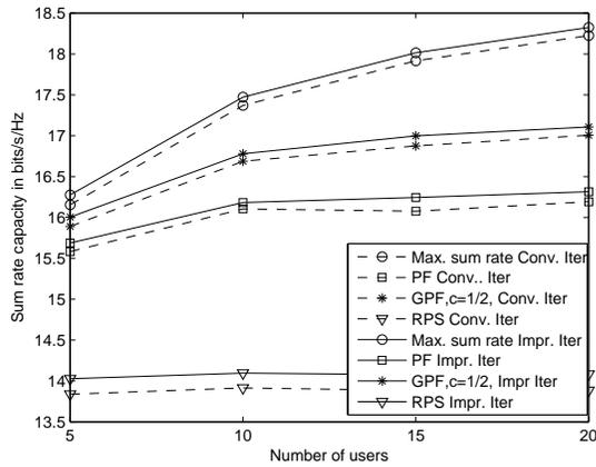
Fig. 5. Performance comparison of the Shannon capacity based scheduling algorithms for the improved iterative IC-MMSE schemes for the QPSK system with  $2 \times 2$  antenna setup. All the curves are plotted at the 3rd iteration when the systems reach convergence, SNR 30 dB.
