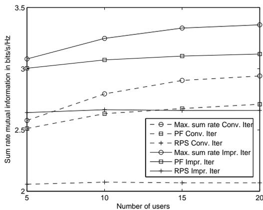
Fig. 2. Performance comparison of the improved and conventional iterative IC-MMSE schemes for the 4ASK system with  $2 \times 2$  antenna setup. All the curves are plotted at the 3rd iteration when the systems reach convergence, SNR 20 dB.
