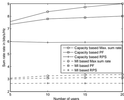
Fig. 3. Sum rate performance comparison for the improved iterative equalizer with MI and capacity based scheduling algorithms for SDM-FDPS MU-MIMO 4ASK systems with  $2 \times 2$  antenna setup, SNR 20 dB.
