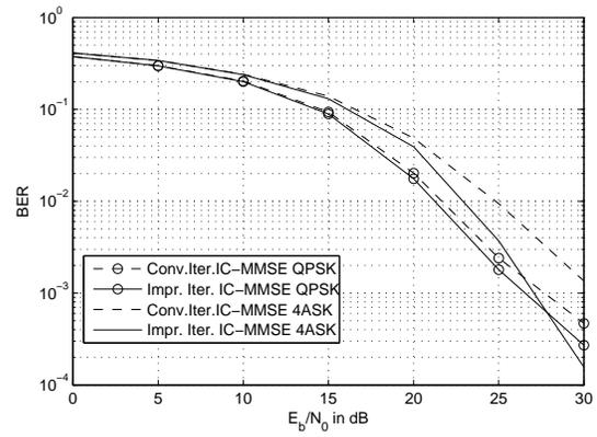
Fig. 7. BER performance of improved iterative receiver scheme with  $4 \times 4$  antenna setup. All the curves are plotted at the 3rd iteration when the systems reach convergence.
