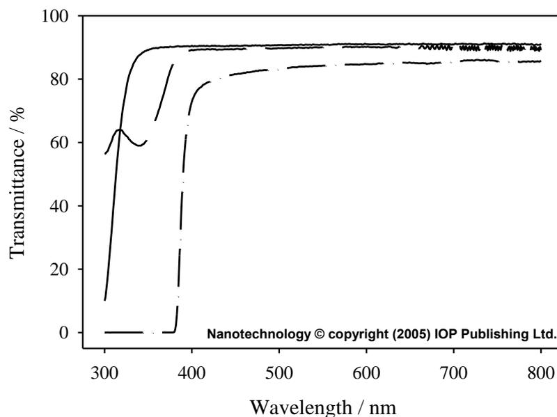
Figure 14. Optical transmission spectra of glass (solid curve), PMMA (dashed curve) and PEN (dash/dot curve) at wavelengths close to the visible region of the electromagnetic spectrum, showing the percentage of visible radiation transmission for each, compared to an air blank, and the near-UV absorption of each sample [99].
