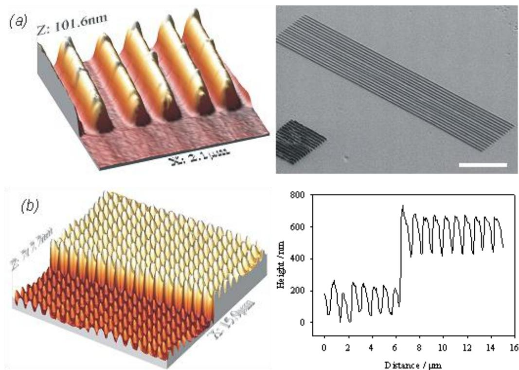
Figure 12. AFM and SEM images of regular nanostructures embossed in PMMA with dimensions of (a) 200 nm wide, 100 nm tall, 80  $\mu\text{m}$  long lines, and (b), 200 nm tall, 1  $\mu\text{m}$  diameter posts embossed on two levels of a 400 nm tall step. The aspect ratio of the lines in the bottom left hand corner of the SEM image in (a) was too high and hence they have collapsed [bar = 5  $\mu\text{m}$ ].
