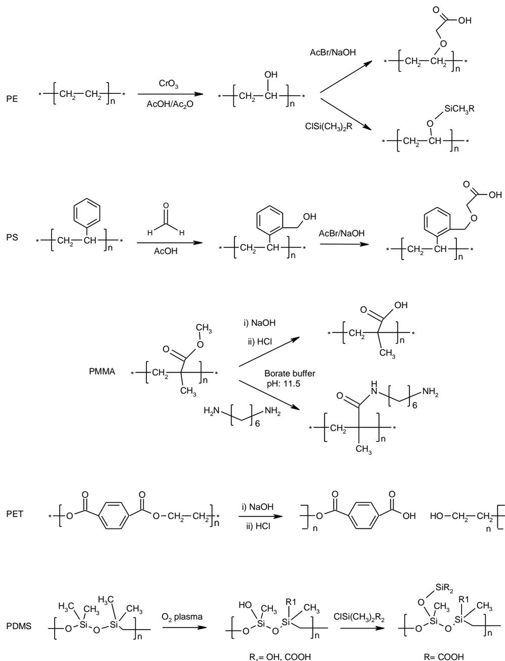
Figure 5. Examples of the surface modification of PE, PS, PMMA, PET and PDMS by chemical means to produce functionalised polymer surfaces with active chemical moieties.
