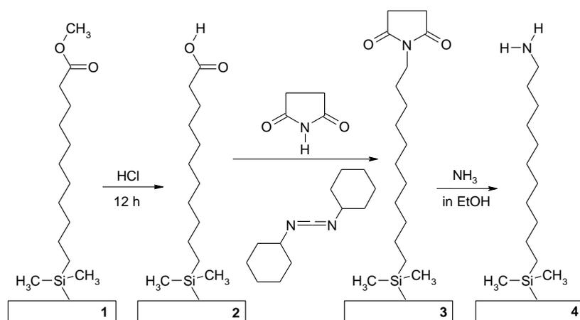
Figure 3. Reaction scheme outlining the chemical transformation of an alkylsilane giving different functional surfaces. These chemical functionalities alter the surface properties of the functionalised substrate surface, for example via a change in hydrophobicity (see figure 4).
