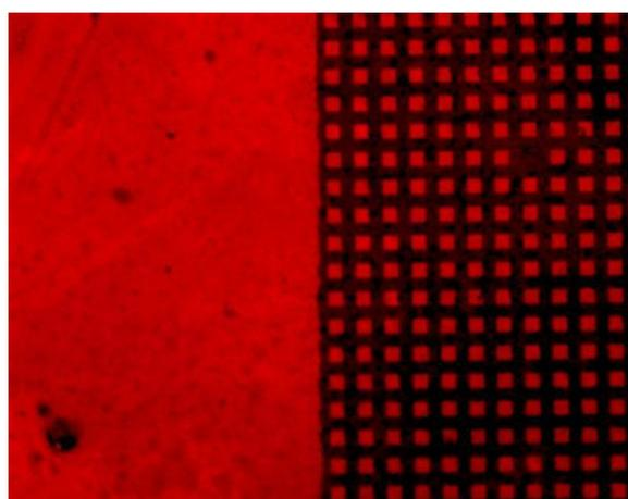
Figure 16. A PMMA surface functionalised with a biotin pattern using a microcontact printing technique. This pattern was subjected to Texas Red dye, and imaged using fluorescence microscopy.
