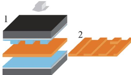
Figure 1. Schematic diagram of the embossing technique used to produce micro/nanostructures in a polymer surface. The polymer is placed in a press, heated to above its  $T_g$ , and embossed under pressure using a stamp with a micro/nanostructured surface (1). The entirety is then cooled to below  $T_g$  before the stamp is removed, leaving the structured polymer surface (2).
