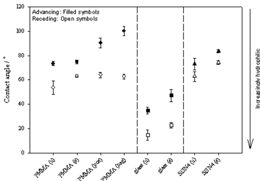
Figure 13. Advancing (filled symbols) and receding (open symbols) water (0.3 ml) contact angle measurements of PMMA surfaces: also shown for comparison are measurements for glass and silicon nitride ( $\text{Si}_3\text{N}_4$ ).
