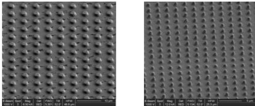
Figure 11. SEM images of regular microstructures, with dimensions of (a) 10  $\mu\text{m}$  diameter, (b) 5 x 5  $\mu\text{m}^2$ , (c) 2.5  $\mu\text{m}$  diameter and (d) 1  $\mu\text{m}$  diameter, and  $\sim$ 400 nm tall, embossed in a 125  $\mu\text{m}$  thick freestanding PMMA sheet, over an area of 1  $\text{cm}^2$ .
