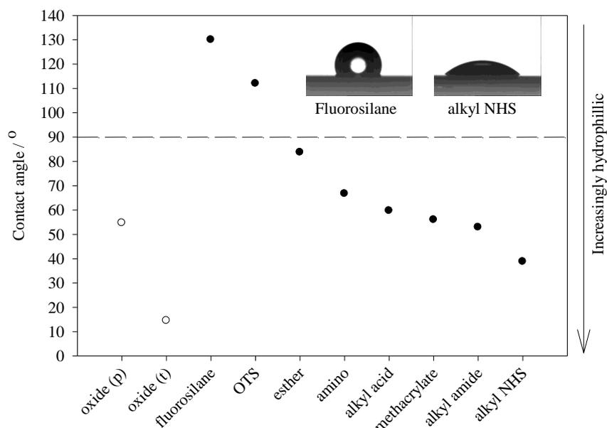
Figure 4. Advancing contact angle measurements of silicon oxide surfaces prior to chemical modification (○) and when functionalised (●). The dotted line indicates the transition from hydrophobic to hydrophilic.
