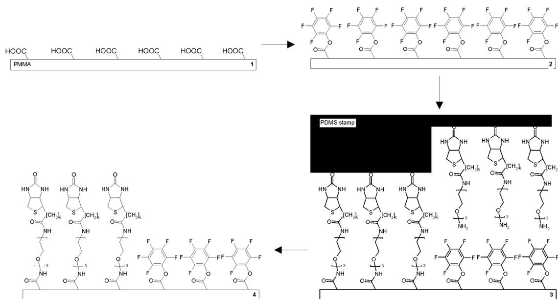
Figure 15. Scheme showing the selective patterning of a PMMA surface with biotin (see text for details).
