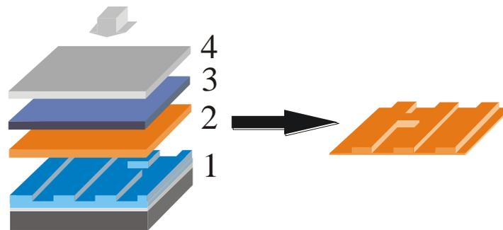
Figure 8. Schematic diagram of the embossing process used to produce freestanding polymer films containing micro/nanostructures. The PMMA (2) is sandwiched between the mould (1) and the aluminium (4) used in the nanoimprinter. The PMMA is protected by a high  $T_g$  polymer (3, see text).
