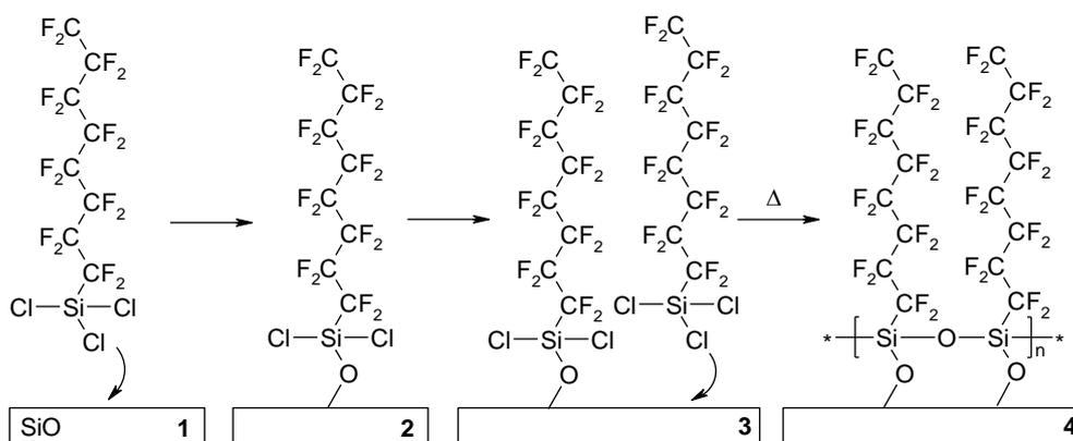
Figure 2. Functionalisation of a silicon surface using trichloro(tridecafluoro-octyl)silane to alter the surface properties; to increase the surface wettability for example (see figure 13).
