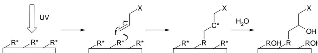
Figure 6. An example mechanism of the grafting of a molecule with a functionalised moiety (X) to a polymer surface.  $R^*$  is an excited moiety on the polymer surface.
