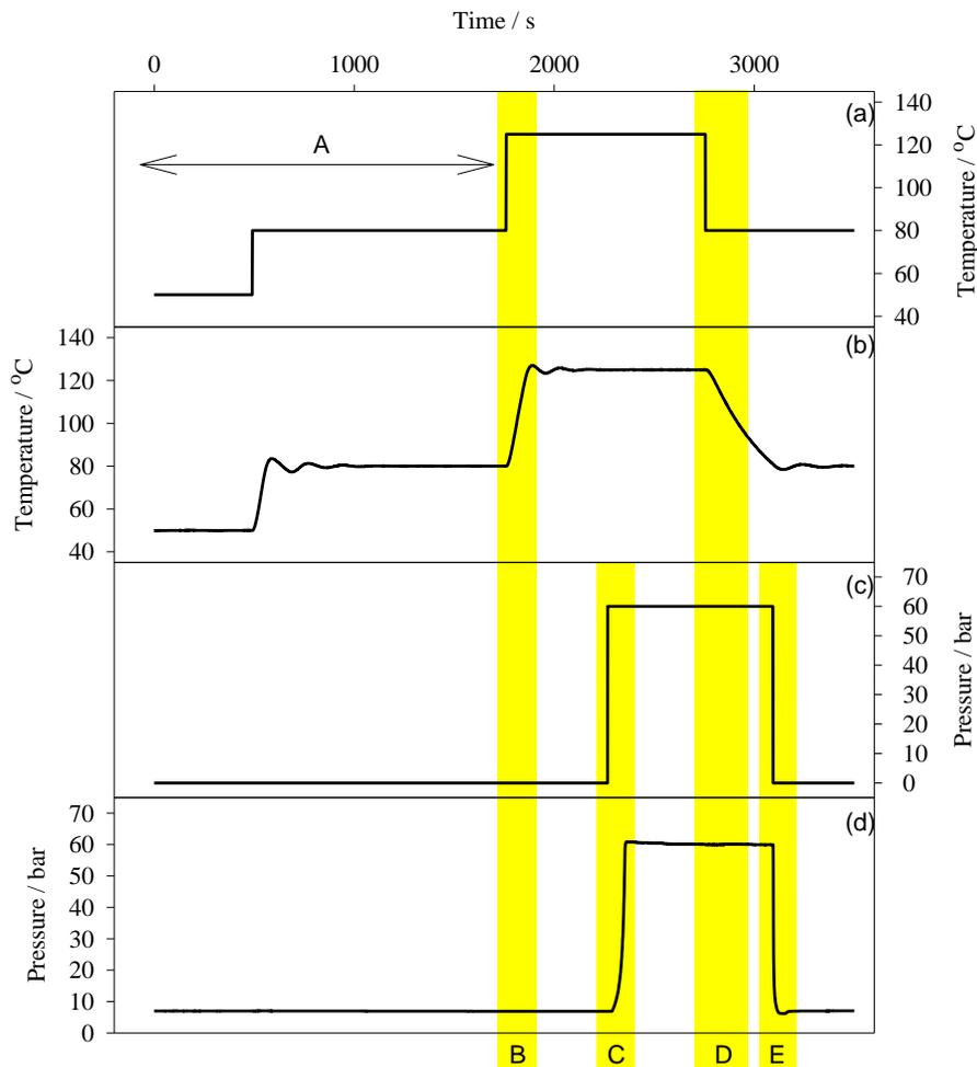
Figure 10. A typical example of a process graph for nanoembossing where (a) is the emperature set point, (b) is the recorded temperature, (c) is the pressure set point, and (d) is the recorded pressure (See text for details).
