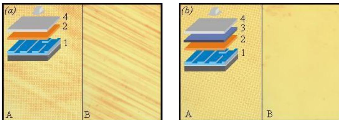
Figure 9. Elimination of backside patterning of 125  $\mu\text{m}$  thick PMMA sheets through the use of a high  $T_g$  polymer layer. In (a) the PMMA (2) is only sandwiched between the mould (1) and the aluminium (4). In (b) the PMMA is protected by the high  $T_g$  polymer (3). In each case, the optical images show the surface
