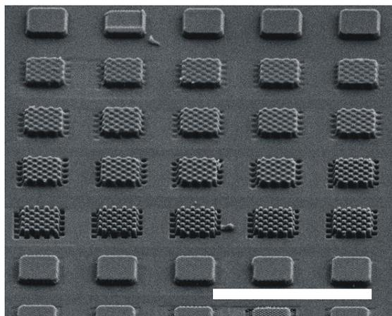
Figure 7. SEM image of a silicon substrate containing 400 nm tall,  $5 \times 5 \mu\text{m}^2$  microstructures, some of which have been modified using FIB milling [bar = 20  $\mu\text{m}$ ].
