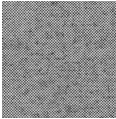
(b) Printed-and-scanned Midtone Grayscale Patch Displayed at Size 256x256 by HP LaserJet4500
