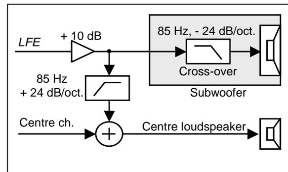
Fig. 2 Simple bass management system used in the experiment.
