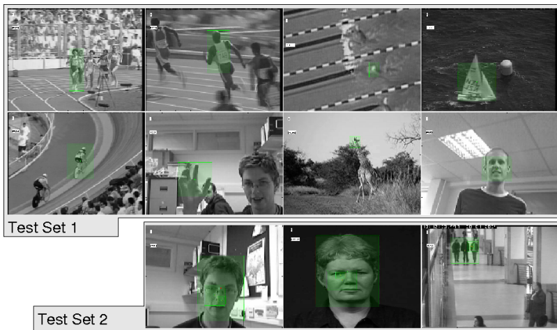
Figure 4: Test sequences used. Set 1 was used to test single feature tracks. Set 2 was used to track 3-tiers of object.
