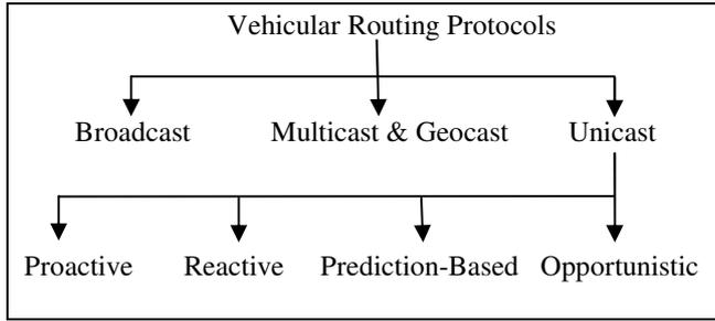
Fig. 5 Categories of vehicular routing protocols
