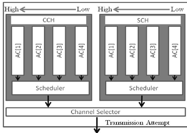
Fig. 4 QoS Queue Structure on a Vehicle in WAVE
