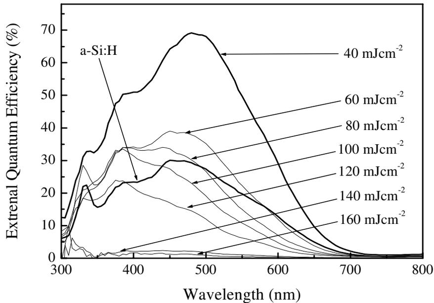
**Figure 3.** External Quantum efficiency of EL crystallised Schottky barrier cells.
