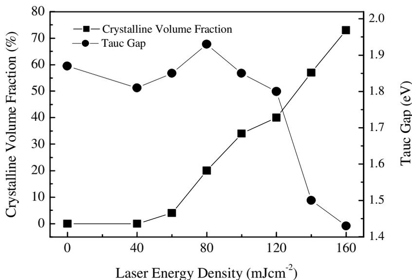
**Figure 2.** Variation of crystalline volume fraction and Tauc gap of EL crystallised silicon with laser energy density.
