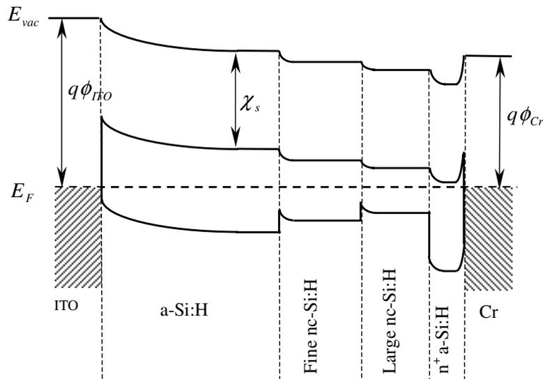
**Figure 2.** Band structure of EL crystallised silicon Schottky barrier cells indicating work functions of ITO (4.7eV) and Cr (4.5 eV) and electron affinity of a-Si:H (4.0 eV).
