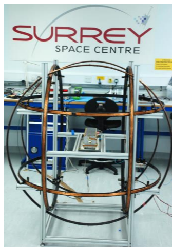
Figure 4. The 3-Axis Helmholtz Coil test facility with AlSat-1N inside
