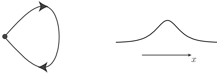
Figure 3: A homoclinic solution to the spatial dynamics formulation (left, shown as a trajectory in phase space) corresponds to a localised solution of the ferrohydrostatic problem (right, sketch of the free surface).
