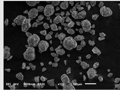
Fig. 3: SEM Image of Alumina
