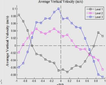
Fig. 12: Radial Time Averaged Velocity
