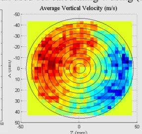
Fig. 7: Time Averaged Vertical Velocity across whole bed height
