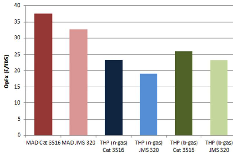
**Figure 7 - Net OpEx comparison with two different CHP units**
