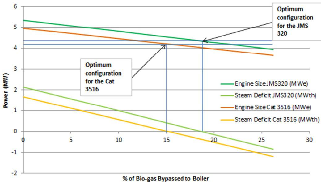
**Figure 8 - Bio-gas bypass with different CHP units**
