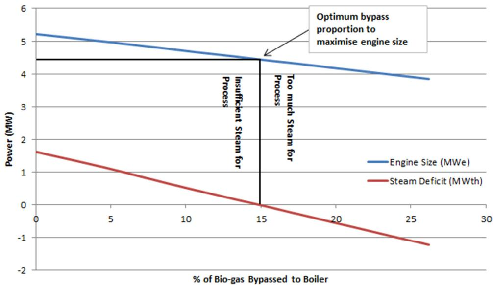
**Figure 5 - Biogas Bypassed and Theoretical Engine Size**
