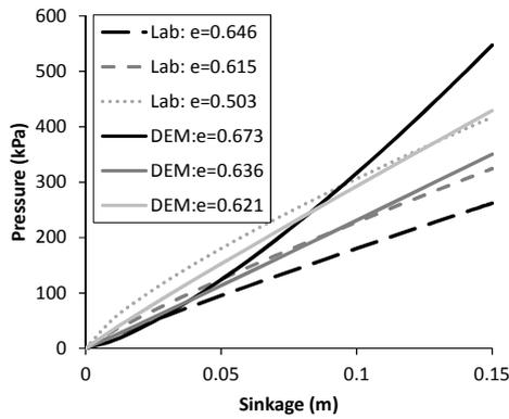
**FIGURE 2.** Bekker's model fit lines for DEM simulations and experimental tests performed by Brunskill et al [7].
