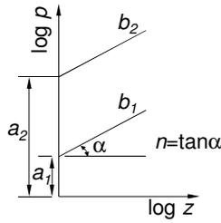
**FIGURE 1.** Illustration of determination of the soil constants in Bekker's model (after [3]).
