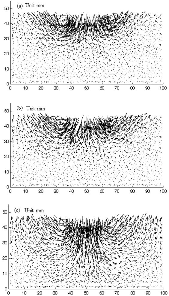
**FIGURE 4.** Particle displacements till the sinkage of 10 mm in the middle section of the specimen with a thickness of 20 mm. (a)  $\mu_{pp}=0.3$ ,  $\mu_{pb}=0.1$ ; (b)  $\mu_{pp}=0.5$ ,  $\mu_{pb}=0.1$ ; (c) rotation prohibited.
