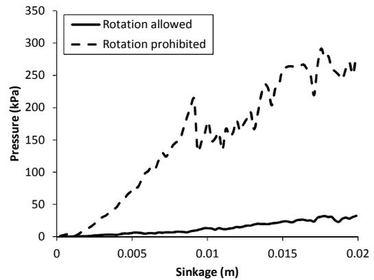
**FIGURE 5.** Comparison of pressure-sinkage relationship for different rolling resistance.
