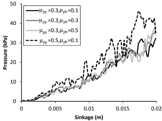
**FIGURE 3.** Comparison of pressure-sinkage relationships for various coefficients of friction.
