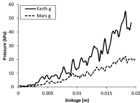
FIGURE 6. Comparison of pressure -sinkage relationships for different gravities.
