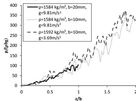
FIGURE 7. Normalised pressure-sinkage relationship.
