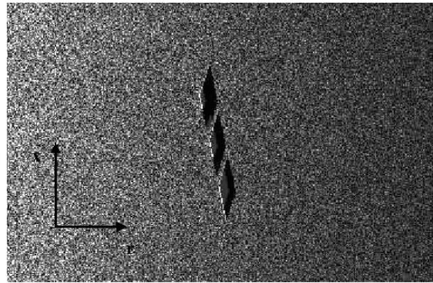
Figure 4. Simulated SAR image relative to three buildings aligned along the direction  $\varphi=40^\circ$ .
