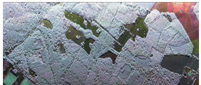
Fig 6. Multipolarimetric airborne S-band image of a forestry area in the UK
