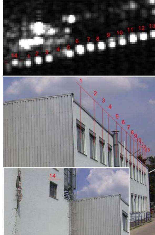
Figure 3. Comparison between SAR image and ground truth. Top: zoom of the short side of the building in the SAR image in Fig.2a; Façade of the short side.
