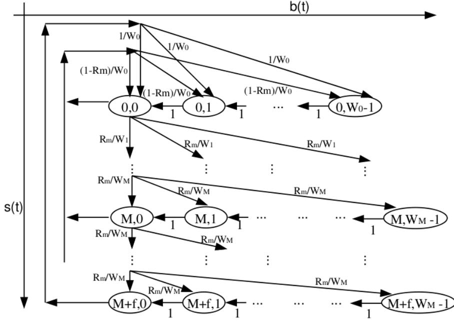
Fig. 3. Two-dimensional Markov chain for a single  $AC_m$ .
