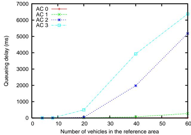
Fig. 14. Queuing delay for each AC in IEEE 802.11p system.
