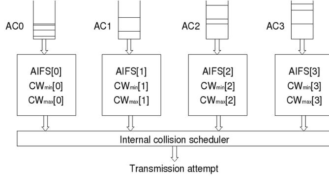
Fig. 1. Prioritization mechanism inside a single STA.
