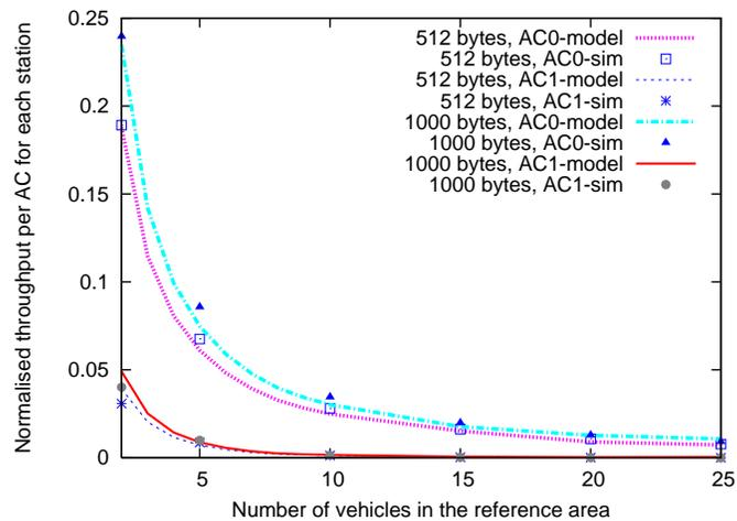
Fig. 9. The impact of packet size on system performance in terms of throughput.
