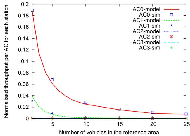
Fig. 8. Normalised average throughput per AC for each station versus the number of vehicles in the reference area.
