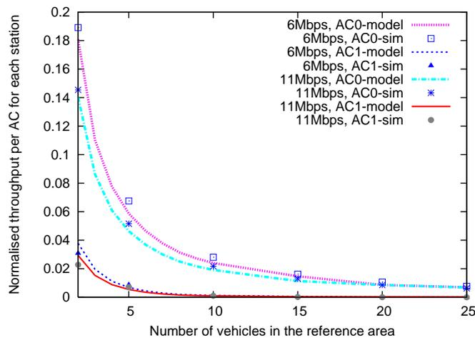
Fig. 10. The impact of channel data rate on system performance in terms of throughput.
