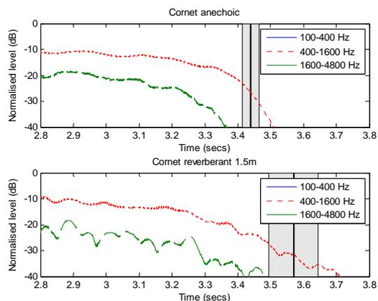
Figure 3: Simple time-energy-frequency analysis of the cornet stimuli, showing the normalised level of the three frequency bands of the anechoic version in the upper plot and the selected reverberant version in the lower plot, over time on the x-axis, scaled to focus on the note offset. The means of the subjective results are shown on each plot as a thick vertical black line, and the associated 95% confidence intervals are shown as a grey area.
