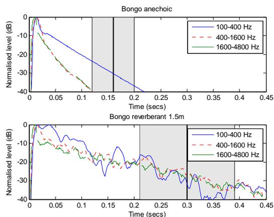
Figure 2: Simple time-energy-frequency analysis of the bongo stimuli, showing the normalised level of the three frequency bands of the anechoic version in the upper plot and the selected reverberant version in the lower plot, over time on the x-axis. The means of the subjective results are shown on each plot as a thick vertical black line, and the associated 95% confidence intervals are shown as a grey area.
