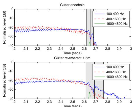
Figure 4: Simple time-energy-frequency analysis of the guitar stimuli, showing the normalised level of the three frequency bands of the anechoic version in the upper plot and the selected reverberant version in the lower plot, over time on the x-axis, scaled to focus on the chord offset. The means of the subjective results are shown on each plot as a thick vertical black line, and the associated 95% confidence intervals are shown as a grey area.
