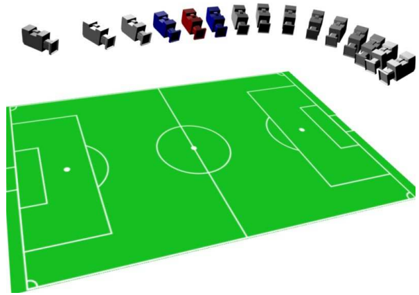
Fig. 10. Arrangement of cameras in soccer stadium. Camera highlighted in red provided ground truth images and was not used for “leave one out” experiment and cameras highlighted in blue were additionally removed for “leave three out” experiment
