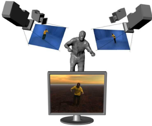
Fig. 1. Free-viewpoint video synthesis: a geometric proxy is used to reproject the appearance sampled in camera images to a new viewpoint.
