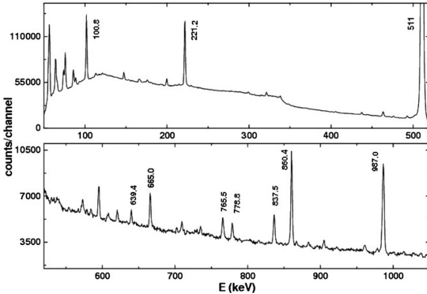
FIG. 1. Total projection  $\gamma$  spectrum obtained in this experiment. All  $\gamma$  lines labeled by their energy in keV belong to the decay of  $^{170}\text{Ta}$  to  $^{170}\text{Hf}$ .
