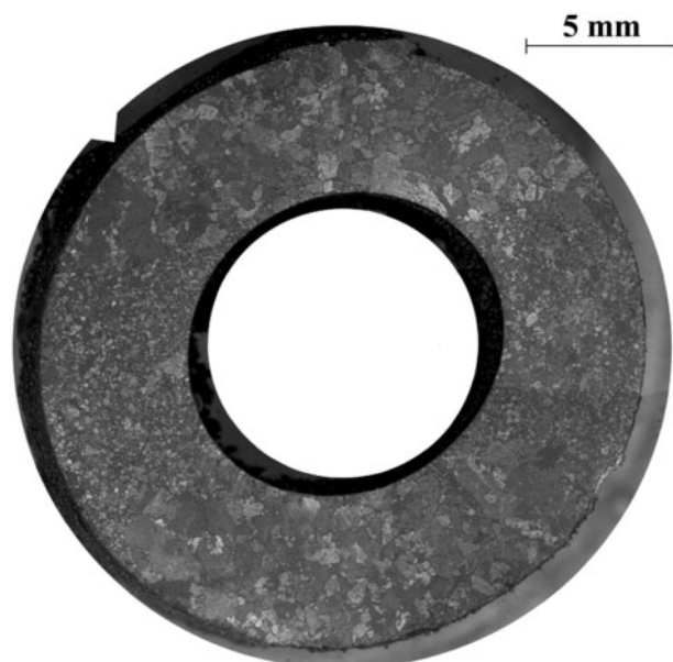
5 Lead pipe sample exhibiting 'zoned' grain structure
