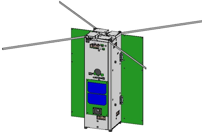
Figure 2. STRaND-1 (with solar panels and antenna deployed)
