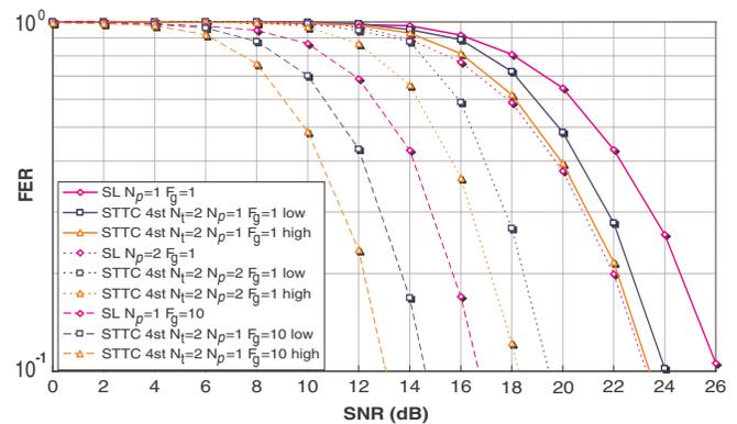
Fig. 3. FER performance comparison of the single link scheme versus the STTC scheme, 4-PPM,  $N_p = 1, 2, P,Q = 1, 10$ , FS-rake-1, 10.
