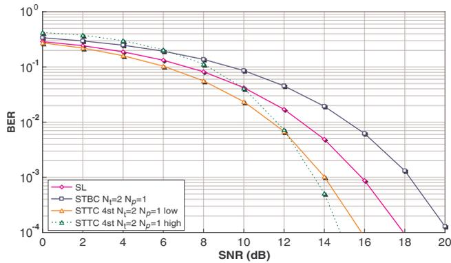
Fig. 2. BER performance comparison of the single link scheme versus the STBC scheme and the STTC scheme, 4-PPM,  $P,Q = 10$ , FS-rake-10.
