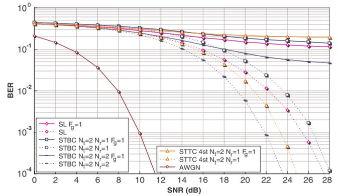
Fig. 1. BER performance comparison of the single link scheme, the STBC scheme, the STTC scheme and AWGN channel, 4-PPM,  $P.Q = 1, 10$ , FS-rake-1.
