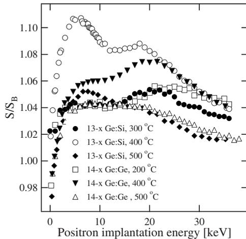
FIG. 5. The low-momentum  $S$  parameter measured at room temperature after 30 min anneal for the set 13- $x$  with Si fluence  $4 \times 10^{14} \text{ cm}^{-2}$  and the set 14- $x$  with Ge fluence  $1 \times 10^{14} \text{ cm}^{-2}$ . The data has been scaled to the parameters measured in bulk Ge with  $S_{\text{Ge}}=0.517$ .
