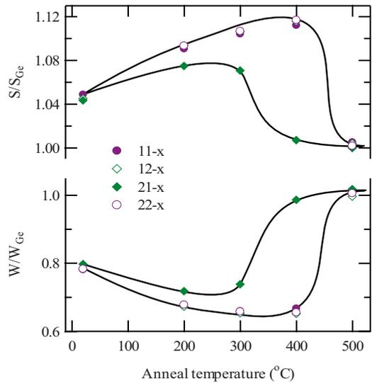
FIG. 3. (Color online) The  $S$  and  $W$  parameter values corresponding to the top of the peak (bottom of the valley) of the  $S$  ( $W$ ) parameter curve as a function of annealing temperature. The data has been scaled to the parameters measured in bulk Ge with  $S_{Ge} = 0.517$  and  $W_{Ge} = 0.036$ .
