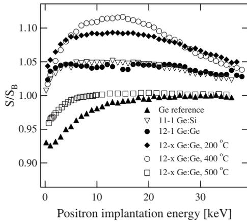
FIG. 2. The low-momentum parameter  $S$  as a function of positron implantation energy for a representative set of as-implanted (fluence  $<10^{14}$  cm $^{-2}$ ) and annealed samples. The data has been scaled to a positron trap free Ge bulk crystal.
