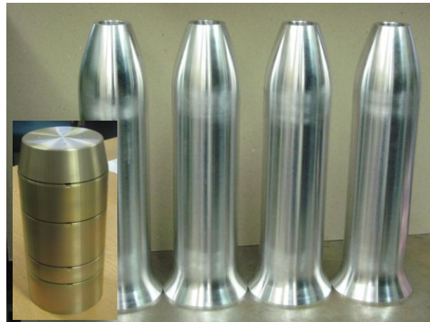
Figure 8: Impact trial penetrator shells and one inner payload bay stack
