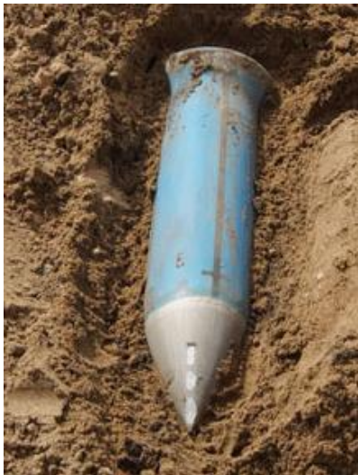
(a) Penetrator-1 resting position in target, showing little rotation; extensive nose but no significant top surface body ablation
