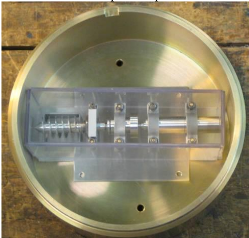
Figure 14: Sample Acquisition Drill Bay (Surrey Space Centre)
