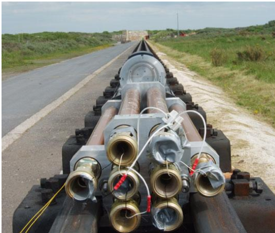
Figure 6: Penetrator mounted in front of rocket-sled with target in the distance
