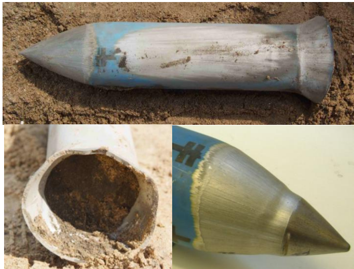
(b) Penetrator shell ablation of nose, underbelly, and tail flare distortion and behind steel nose of 3 rd penetrator
