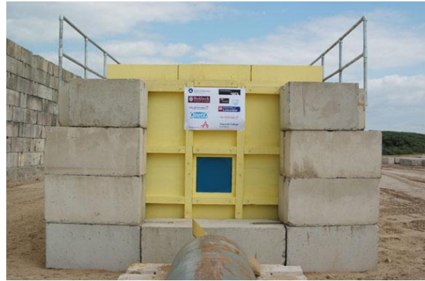
Figure7: Impact target showing entrance aperture. In the foreground at the bottom is a tube which catches the sleds.
