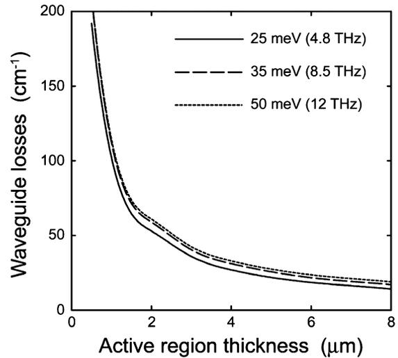
Fig. 10. Plot showing the waveguide losses against active region thickness on top of a 400-nm WSi<sub>2</sub> reflector for three different frequencies.
