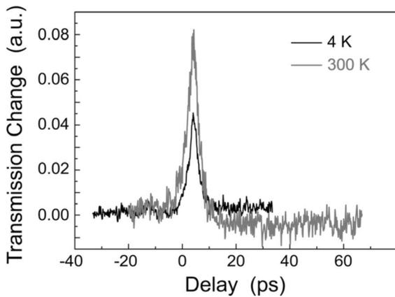
Fig. 6. Differential probe transmission against optical delay for two temperatures for the LH1-to-HH1 intrawell lifetime at 32.9 meV (7.90 THz).
