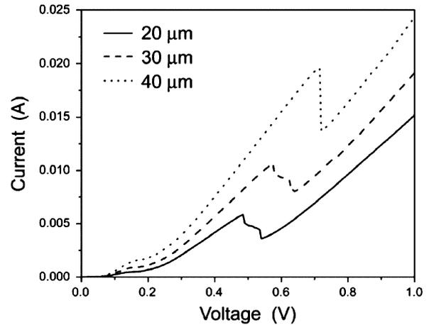
Fig. 2. Current versus voltage for three different RTD devices with different areas. Current peak corresponds to the tunneling between the contacts and the HH2 states in the quantum well.
