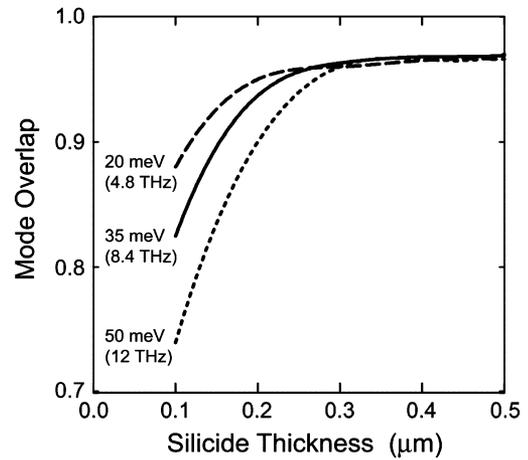
Fig. 9. Plot showing the mode overlap against buried silicide (WSi<sub>2</sub>) thickness for a 4- $\mu\text{m}$  active region at three different frequencies.
