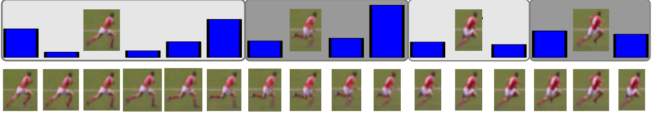
Figure 4. An animation summary. The bottom row is the original animation. The top row shows the key-frames in the summarised representation. The gray boxes indicate the frames of the animation represented by each key-frame. The blue bars above each frame are a plot of the distortion introduced by representing the frame with the respective key-frame.
