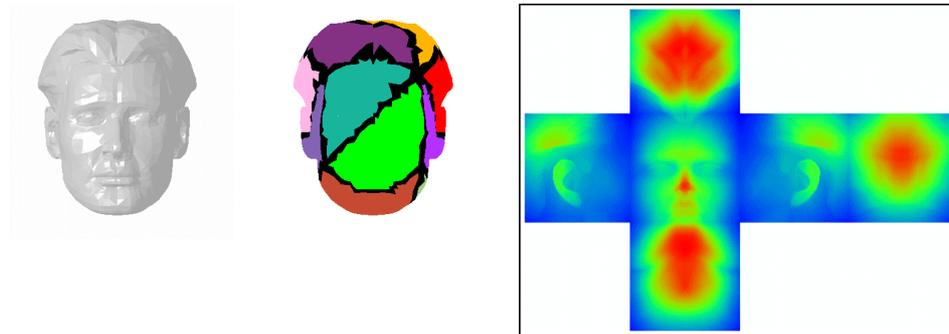
a) Captured Shape      b) Mapping to Cube      c) Displacement map image
